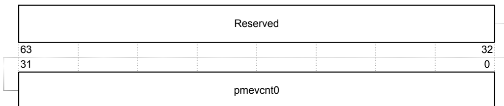
Figure 3-102 pmevcnt0 register bit assignments
